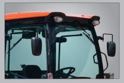
**Standard Front & Rear Wipers** The front and rear window wipers ensure the clear visibility by keeping the window clean from rain, dust or condensation. Wipers are positioned to minimize the impact on operator's view.
