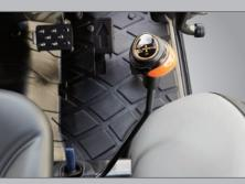
**Single Lever Joystick** Front end loader work is made easier by the use of a single lever joystick. The lever returns to neutral when released. A float position allows the bucket free flotation over the ground surface.
