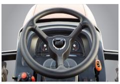
Power Steering with Tilt The standard power steering minimizes the effort required to make tight, repetitive turns. The steering wheel tilts to adjust for operator needs.
